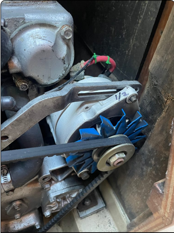
Upgraded alternator and 1/2" belt
