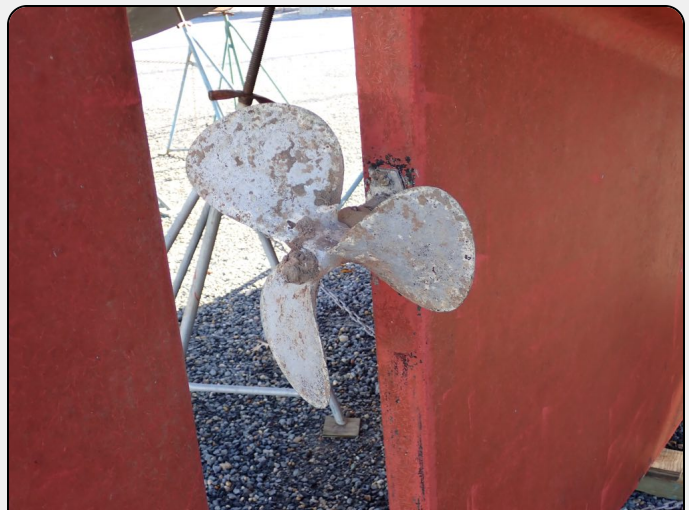
Propeller shows no signs of damage but should be cleaned and conditioned as needed.
