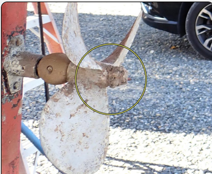
Propeller nut area showing fouling
