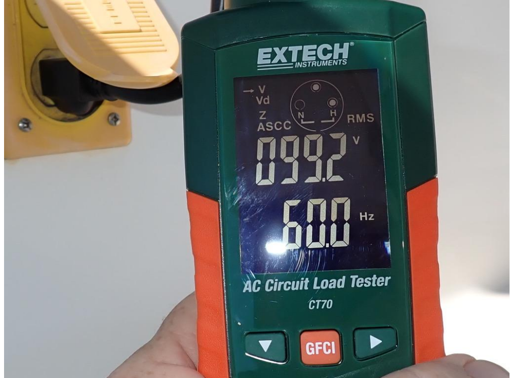
Reverse Polarity at the Outlet
