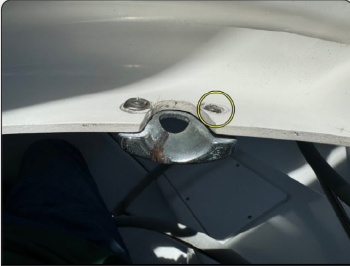
screw head pulled through; add washer and refasten
